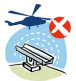
**SWITCH OFF** the radar once the helicopter is overhead.
