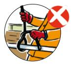
**DO NOT SECURE** the winch wire to the vessel.
